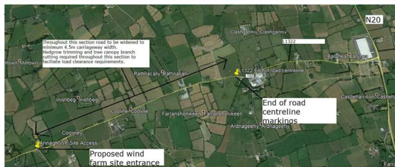
**KEY PLAN: L1322 CONSTRAINED SECTION BETWEEN NODE 10.5 and PROPOSED SITE ENTRANCE**
